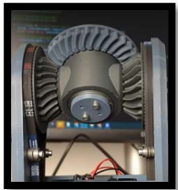
Figure 7 - Multi Directional Movement using 1 Motor
